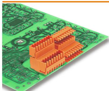
Double-level, staggered pin header for wave soldering at 3.50 mm pitch. They are available in closed and flanged versions. The male connectors provide space for labelling and can be coded.
