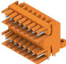
Two-tier pin header for wave soldering in 3.50 mm pitch. The connector is available in open, closed and flange versions. The male connectors provide space for labelling and can be coded. Packed in a cardboard box.
