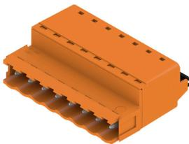
Male plug with PUSH IN wire connection and straight outlet direction, when used with BLF 5.08HC as wire-to-wire application for panel feed-through The male plugs provide space for labelling and can be coded.
