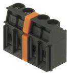
The maximum voltage is based on the minimum distance. Intermediate plates increase the creepage and clearance distances between different potentials and permit higher rated voltages or a clear separation, e.g. between mains and low voltages or different protection zones.
