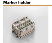
The marker holder offer the possibility of additional mounting of standard markers with a pitch of 5 or 5.1 mm. The angled holders can be optionally snaped together and could be mounted in all standard marking channels of the Klippon® Connect modular terminal blocks. Fitting marker types could be found under the respective accessories of the designation marking holder.
