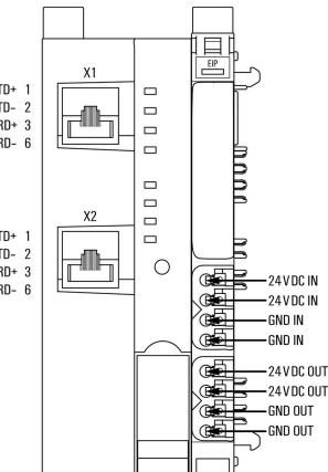
**Explanation of abbreviations****Field bus coupler**
