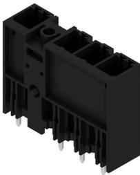
180° male header with middle flange with a 7.62 pitch. Meets the requirements of IEC 61800-5-1 and enables UL approval as per UL840 600 V. Without a female header, the mating profile guarantees minimum touch safety of >3 mm with 20 N pressure on the test finger.
