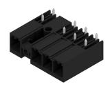
270° male header with middle flange with a 7.62 pitch. Meets the requirements of IEC 61800-5-1 and enables UL approval as per UL840 600 V. Without a female header, the mating profile guarantees minimum touch safety of >3 mm with 20 N pressure on the test finger. The automatically locking middle flange which can optionally also be screwed, reduces space requirements by one pitch width in comparison with conventional solutions.
