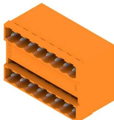
2-tier male header with parallel pin arrangement. The solder pin length is optimised for wave flow soldering. The pin headers provide space for labelling and can be coded.
