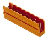
Male connectors with straight outlet direction. The solder pin length is optimised for wave flow soldering. The pin headers provide space for labelling and can be coded.
