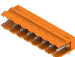
Male connectors with 90° outlet direction. The solder pin length is optimised for wave flow soldering. The pin headers provide space for labelling and can be coded.
