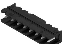
High-temperature-resistant, 90° angled, open male header. Packed in box or tape. On tape, with 1.5 mm solder pin, optimised for automatic assembly. 3.2 mm solder pin suitable for reflow and wave soldering. The pin headers provide space for labelling and can be coded. HC = High Current.
