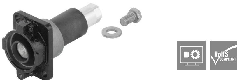
The protective housing is manufactured from seawater-resistant aluminium using pressure die casting. High standards of water and dust protection, as well as particularly high impact resistance, are the hallmarks of this housing series. A sophisticated two-stage surface coating ensures years of reliability. All screws, crimp contacts and other exterior accessory parts are made of corrosion-resistant stainless steel.
