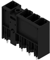
180° male header with middle flange with a 7.62 pitch. Meets the requirements of IEC 61800-5-1 and enables UL approval as per UL840 600 V. Without a female header, the mating profile guarantees minimum touch safety of >3 mm with 20 N pressure on the test finger. The automatically locking middle flange which can optionally also be screwed, reduces space requirements by one pitch width in comparison with conventional solutions. On request: available with screw flange or without flange.
