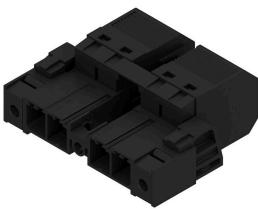
180° inverted male header with PUSH IN connection technology for field wiring in 6 mm<sup>2</sup> with 7.62 pitch as "three-flange variant" for housing passage. Suitable for housings with a max. wall thickness of 2 mm. Also perfect as a finger-safe solution for inverse voltages. Meets the requirements of UL1059 600 V class C and IEC 61800-5-1.
