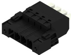
180° inverted pin header with PUSH IN connection technology and adjustable actuator (pusher) for field wiring 6 mm<sup>2</sup> in a 7.62 pitch. Also ideal as a touch-safe solution for inverse voltages. Meets the requirements of UL1059 600 V Class C and IEC 61800-5-1. Variants: without flange, external flange, middle flange with snap-on mechanism and optional additional screw mount.
