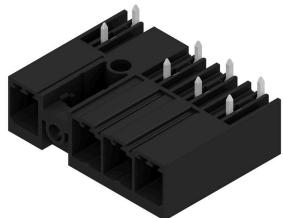
270° male header with middle flange with a 7.62 pitch. Meets the requirements of IEC 61800-5-1 and enables UL approval as per UL840 600 V. Without a female header, the mating profile guarantees minimum touch safety of >3 mm with 20 N pressure on the test finger. The automatically locking middle flange which can optionally also be screwed, reduces space requirements by one pitch width in comparison with conventional solutions. On request: available with screw flange or without flange.
