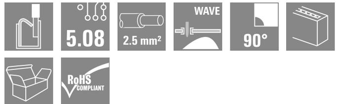
The new LMF allows us to meet the current market requirements for a PCB terminal with PUSH IN connection system for wire cross-sections up to 2.5 mm<sup>2</sup>
