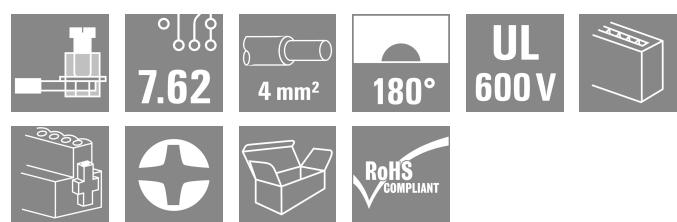
180° female plug with a 7.62 pitch for IT power networks. Meets the requirements of UL1059 600 V class C. In combination with male header SL 7.62 IT.... With leading contact. Meets the extended requirements on 5.5 mm touch safety for IT power networks as per IEC 61800-5-1 for 400 V to earth. The self-locking middle flange which can optionally be screwed, reduces space requirements by one pitch width in comparison with conventional solutions.
