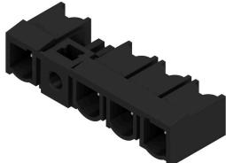
90° male header with soldered flange fastening with 7.62 pitch for 400 V IT power networks according to IEC 61800-5-1. UL approval as per UL840 600 V with leading PE contact.
