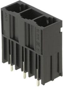
Single-row, high-current male header, for side-by-side mounting without sacrificing any poles, or with patented flange for fast locking without tools. Maximum connection and operating reliability thanks to a mating profile that prevents incorrect connection, with unique coding diversity, additional fastening and integrable positioning aid. 3.5 mm pin length is optimised for wave soldering, plug-in direction 180° to solder pins.
