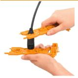
With the multi-tool, Weidmüller is offering a multifunctional tool for processing PV solar connectors.
