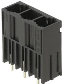
Single-row, high-current male header, for side-by-side mounting without sacrificing any poles, or with patented flange for fast locking without tools. Maximum connection and operating reliability thanks to a mating profile that prevents incorrect connection, with unique coding diversity, additional fastening and integrable positioning aid. 3.5 mm pin length is optimised for wave soldering, plug-in direction 180° to solder pins.
