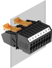
The PGK 4 device feed-through terminal is the fastest and most compact solution for feed-throughs in housings. The innovative PUSH IN connection system from Weidmüller makes for a simple, tool-free wire connection on the inside and outside of devices. The sliced design and an intuitive fastening mechanism enable high-density blocks to be constructed quickly and easily.
