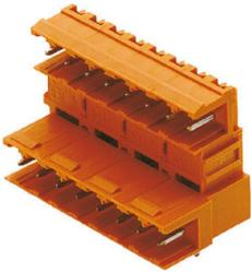
Dimensionally stable, angled, codable 2-tier male connector from the Unimate range of plugs with integral aid to prevent wrong connections. Available with open or closed sides. Fixing blocks can be attached to the closed version. The solder pin length of 3.2 mm has been optimised for wave soldering. Supplied in cardboard box.
