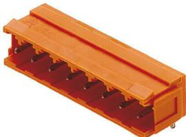
Dimensionally stable, angled, codable male connector from the Unimate range of plugs with integral aid to prevent wrong connections. Available with open or closed sides. Fixing blocks can be attached to the closed version. The solder pin length of 3.2 mm has been optimised for wave soldering. Supplied in cardboard box.
