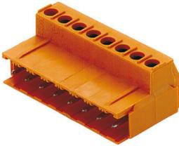
Male header with screw conductor connection for flying leads. Clip-on feet for mounting on the terminal rail and fixing blocks are available for this male connector with clamping yoke connection. The SLAS provides space for labelling and can be coded. Supplied in cardboard box.
