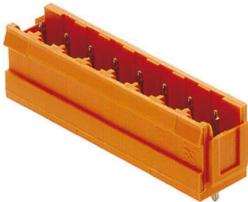
Dimensionally stable, straight, codable male connector from the Unimate range of plugs with integral aid to prevent wrong connections. Available with open or closed sides. Fixing blocks can be attached to the closed version. The solder pin length of 3.2 mm has been optimised for wave soldering. Supplied in cardboard box.
