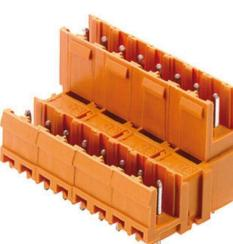
Dimensionally stable, straight, codable 2-tier male connector from the Unimate range of plugs with integral aid to prevent wrong connections. Available with open or closed sides. Fixing blocks can be attached to the closed version. The solder pin length of 3.2 mm has been optimised for wave soldering. Supplied in cardboard box.
