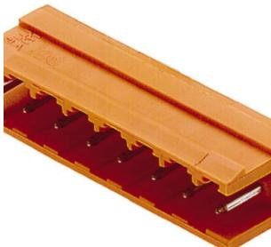
Dimensionally stable, angled, codable male connector from the Unimate range of plugs with integral aid to prevent wrong connections. Available with open or closed sides. Fixing blocks can be attached to the closed version. The solder pin length of 3.2 mm has been optimised for wave soldering. Supplied in cardboard box.
