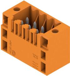
Straight, double-row pin header available in closed-sided or flange version (open-sided pin headers on request). The male headers with a pin length of 3.5mm are designed for wave soldering and are packed in a box. They can be screwed on to the PCB. The male headers provide space for labelling and can be coded.
