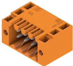
Angled, two-tier pin header available as closed-sided or with flange (open-sided pin headers on request). Pin headers with 3.5mm pins are designed for wave soldering and are packaged in a box. They can be screwed on to the PCB. The pin headers provide space for labelling and can be coded.
