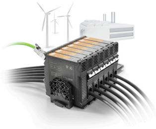
The ACT20C series was especially developed for applications with continuous processes. It enables the continuous monitoring of diagnostic, device and process information ("condition monitoring"). Several ACT20C components form a station which consists of an ACT20C Ethernet gateway, communicative ACT20C signal converters and an ACT20C bus termination terminal.
