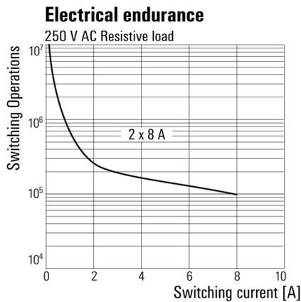
Electrical service life 250 V AC resistive load
