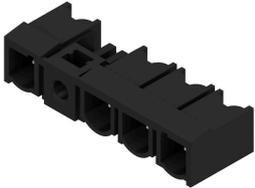
90° male header with soldered flange fastening with 7.62 pitch for 400 V IT power networks according to IEC 61800-5-1. UL approval as per UL840 600 V with leading PE contact.
