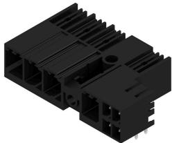
Combined 90° male header with power and signal contacts in PUSH IN connection technology incl. self-locking middle flange interlock and (optional) pluggable shield connection with a 7.62 pitch.
