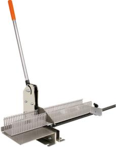
Wire channel cutter for manual operation in cutting wiring channels and covers up to 125 mm wide and a wall thickness of 2.5 mm. Only for plastics not reinforced by fillers.
