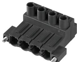
180° inverted male header with clamping yoke connection for field wiring in 2.5 mm<sup>2</sup> with a 7.62 pitch. Also ideal as a touch-safe solution for inverse voltages. Meets the requirements of UL1059 600 V class C and IEC 61800-5-1.
