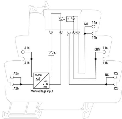
\*Contact is assembled in socket but not used with solid-state relays
