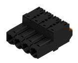
180° inverted male header with PUSH-IN connection technology for field wiring in 2.5 mm² with a 7.62 pitch. Also ideal as a touch-safe solution for inverse voltages. Meets the requirements of UL1059 600 V class C and IEC 61800-5-1.
