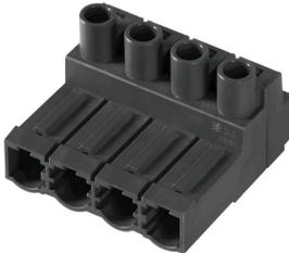
180° inverted male header with clamping yoke connection for field wiring in 2.5 mm<sup>2</sup> with a 7.62 pitch. Also ideal as a touch-safe solution for inverse voltages. Meets the requirements of UL1059 600 V class C and IEC 61800-5-1.
