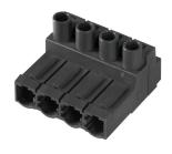
180° inverted male header with clamping yoke connection for field wiring in 2.5 mm² with a 7.62 pitch. Also ideal as a touch-safe solution for inverse voltages. Meets the requirements of UL1059 600 V class C and IEC 61800-5-1.
