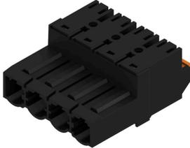
180° inverted male header with PUSH-IN connection technology for field wiring in 2.5 mm<sup>2</sup> with a 7.62 pitch. Also ideal as a touch-safe solution for inverse voltages. Meets the requirements of UL1059 600 V class C and IEC 61800-5-1.
