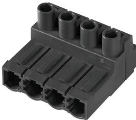
180° inverted male header with clamping yoke connection for field wiring in 2.5 mm<sup>2</sup> with a 7.62 pitch. Also ideal as a touch-safe solution for inverse voltages. Meets the requirements of UL1059 600 V class C and IEC 61800-5-1.
