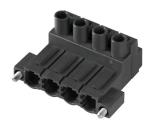
180° inverted male header with clamping yoke connection for field wiring in 2.5 mm² with a 7.62 pitch. Also ideal as a touch-safe solution for inverse voltages. Meets the requirements of UL1059 600 V class C and IEC 61800-5-1.
