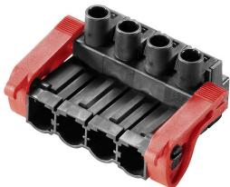
180° inverted male header with clamping yoke connection for field wiring in 2.5 mm<sup>2</sup> with a 7.62 pitch. Also ideal as a touch-safe solution for inverse voltages. Meets the requirements of UL1059 600 V class C and IEC 61800-5-1. Variants: available without flange, with external flange or with release latch.
