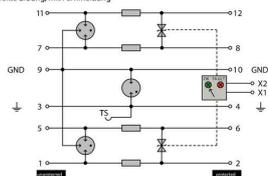
Complete module indirect grounding, with remote signalling
