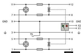
Complete module direct grounding, with remote signalling
