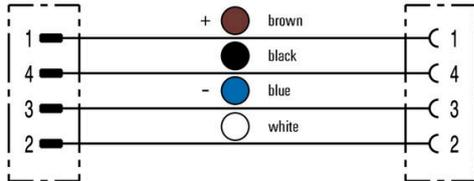
Light, securely screwed-in round plug-in connectors. Screwty set DM / VPE: 1 / Order No.: 1920000000 Adapters: M12, M12 F, M8, M8 F
