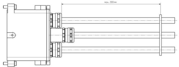
To avoid damage to the contacts and insulating sleeves, we recommend fixing the cable. The corresponding distances are shown in the following drawing. The cable fixation is not included in the scope of delivery.
