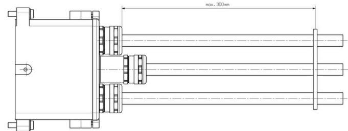
To avoid damage to the contacts and insulating sleeves, we recommend fixing the cable. The corresponding distances are shown in the following drawing. The cable fixation is not included in the scope of delivery.
