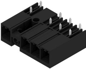
270° male header with middle flange with a 7.62 pitch. Meets the requirements of IEC 61800-5-1 and enables UL approval as per UL840 600 V. Without a female header, the mating profile guarantees minimum touch safety of >3 mm with 20 N pressure on the test finger.
