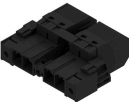
180° inverted male header with PUSH IN connection technology for field wiring in 6 mm<sup>2</sup> with 7.62 pitch as "three-flange variant" for housing passage. Suitable for housings with a max. wall thickness of 2 mm.
