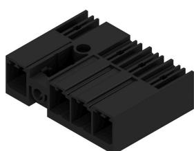
90° male header with middle flange with a 7.62 pitch. Meets the requirements of IEC 61800-5-1 and enables UL approval as per UL840 600 V. Without a female header, the mating profile guarantees minimum touch safety of >3 mm with 20 N pressure on the test finger. The automatically locking middle flange which can optionally also be screwed, reduces space requirements by one pitch width in comparison with conventional solutions. On request: available with screw flange or without flange.
