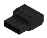
180° inverted pin header with PUSH IN connection technology for field wiring in 6mm² in a 7.62 pitch, as a "three-flange variant" for enclosure feed-through. Suitable for enclosures with a max. wall thickness of 2mm. Also perfect as a touch-safe solution for reverse voltages. Meets the requirements of UL1059 600 V Class C and IEC 61800-5-1.
