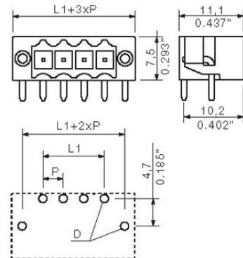
$L1 = 52.50 \text{ mm}$  |  $P = 3.50 \text{ mm}$
