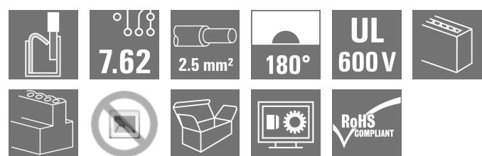
180° inverted male header with PUSH-IN connection technology for field wiring in 2.5 mm<sup>2</sup> with a 7.62 pitch. Also ideal as a touch-safe solution for inverse voltages. Meets the requirements of UL1059 600 V class C and IEC 61800-5-1. Variants: available without flange, with external flange, with release latch.
