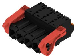
180° inverted male header with PUSH-IN connection technology for field wiring in 2.5 mm<sup>2</sup> with a 7.62 pitch. Also ideal as a touch-safe solution for inverse voltages. Meets the requirements of UL1059 600 V class C and IEC 61800-5-1.
