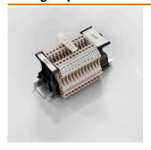
The SchT 5 S group tag carriers are clipped directly onto the TS 32 mounting rail (G-rail) or the TS 35 mounting rail (top-hat rail). It is therefore possible to label the terminal strip irrespective of the terminal and the type of terminal. SchT 5 and SchT 5 S are fitted with ESO 5, STR 5 protective strips.
