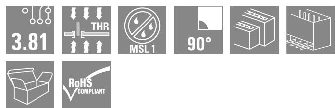
Extra flat high-temperature-resistant two-tier SCDN-THR pin header for reflow soldering.
