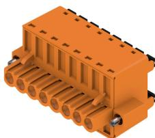
The powerful daisy-chain solution for high-performance signal bus applications is also suitable for 400V auxiliary power chains with 18.5A current-carrying capacity. The large clamping capacity (up to 2.5mm<sup>2</sup> wire cross-sections) is particularly beneficial for long bus cables or high currents because of the low voltage drop. Four flange variations, including the patented release latch, allow for user-friendly unplugging designs.
