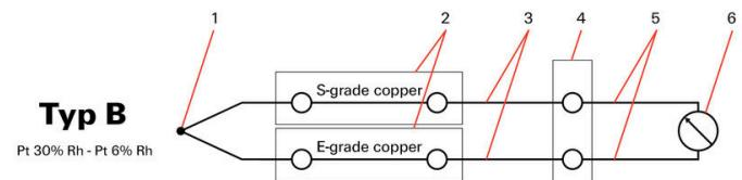
1. Thermocouple (sensor)
