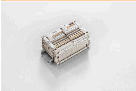
The ZGB 15 is a hinged group tag carrier. The tag carrier can hold the dekafix 5, WS 12/5 terminal markers or the inlay tag ESO 15.
